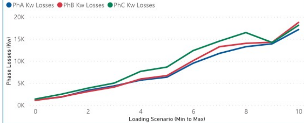
Substation Kw Loss Distribution by Scenario
